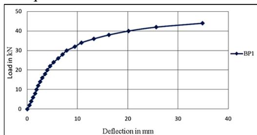
Figure 4.6 Load-deflection behaviour of perfect beam (series 1)
