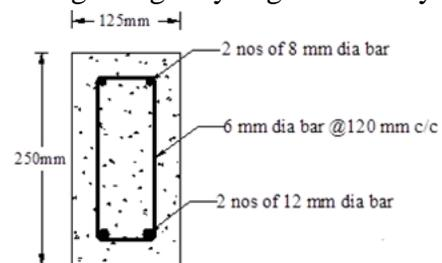
Figure 4.3 Cross section of the beam
