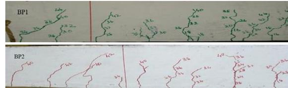
Figure 4.7 Crack patterns of perfect beams (series 1)
