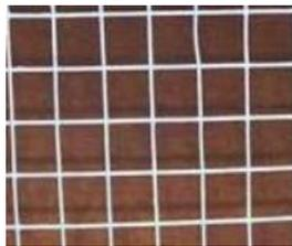
Figure 4.1 Welded wire mesh
