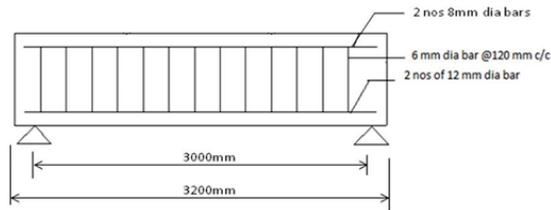
Figure 4.4 Longitudinal section of the beam
